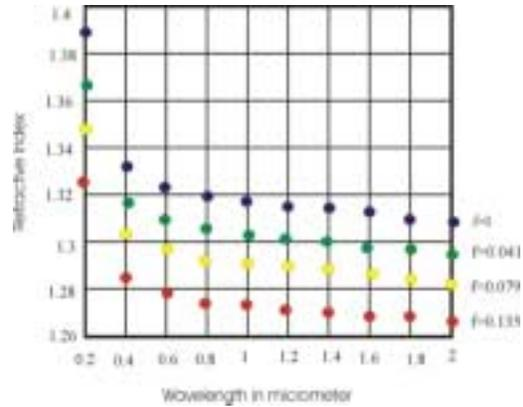
Fig.2: Effect of boron doping on refractive index of pure silica.
