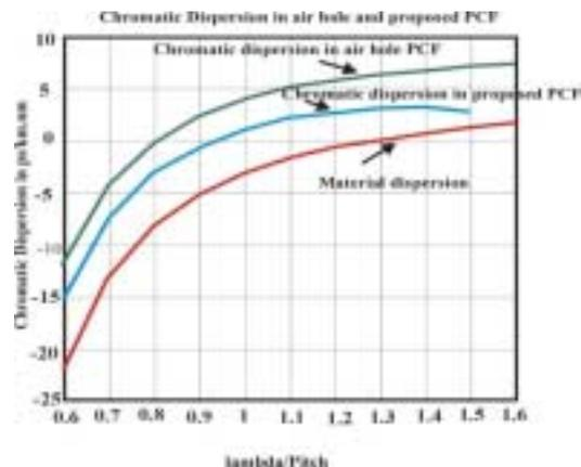
Fig. 6: Chromatic dispersion in air hole and proposed PCF for  $d/\Lambda$  value of 0.4
